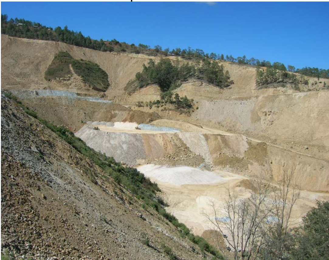
PHOTO 22 – Waste Rock Facility (WRF) being developed in benches from bottom up
