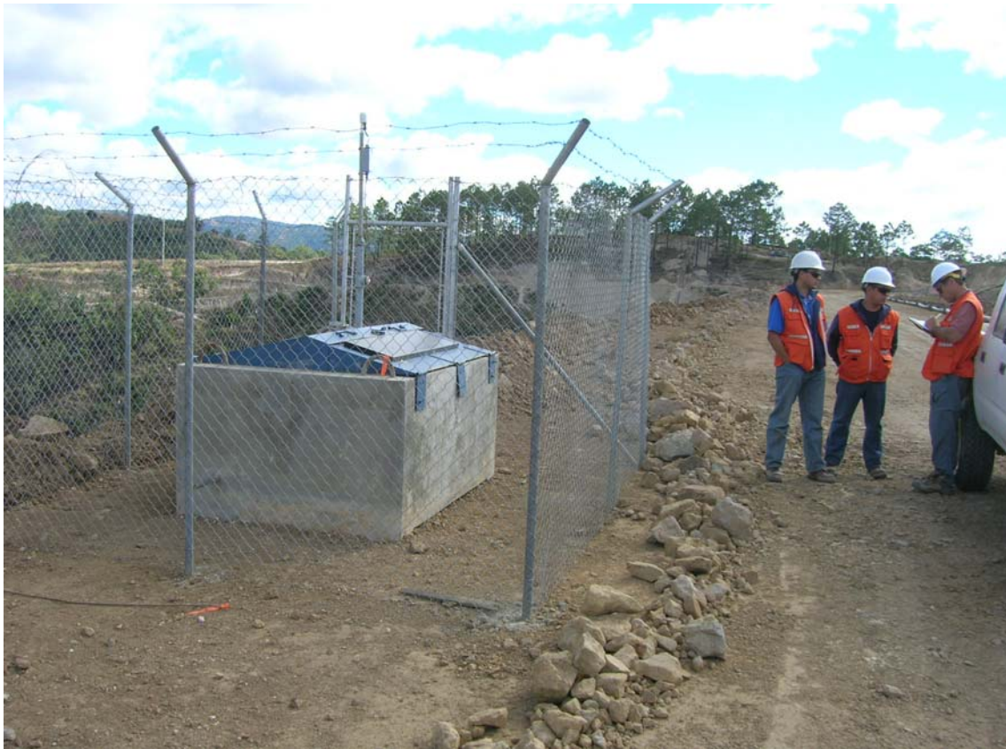
Photo 7 – Container housing seismometer on dam crest
