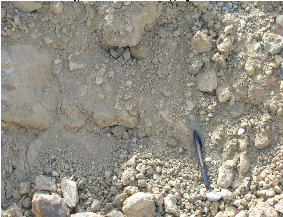
PHOTO 14 – High fines content of d/s rockfill
