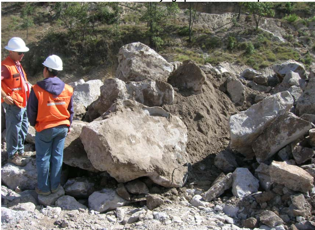
Photo 12 – Large boulders and sand fines in rockfill
