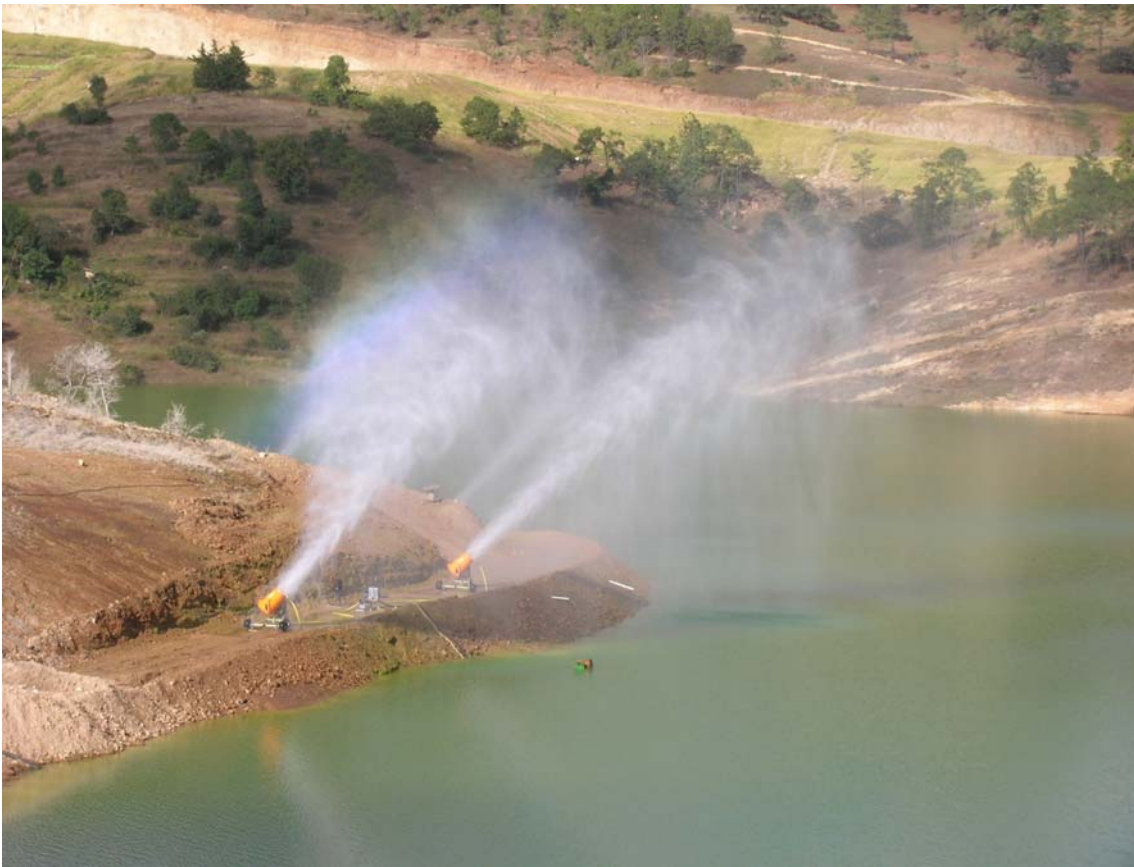
PHOTO 3 – Vaporizing tailings water to reduce water accumulation
