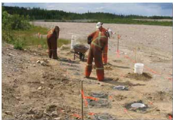
Re-vegetation test plots were installed near the tailings impoundment area during the summer. Each pail holds desulphurized tailings generated during the pilot study conducted for the removal of sulphide minerals from Musselwhite Mine tailings. When fully operational in 2008, the test plots will be prepared with various depths of growth medium then planted with combinations of trees and grasses. Soil and plant combinations will be used to
